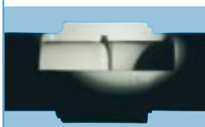
Socket fusion – the connection for smaller dimensions
