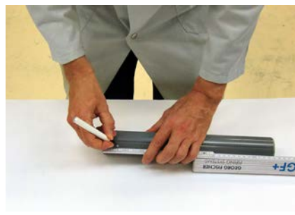
Marking the jointing length
