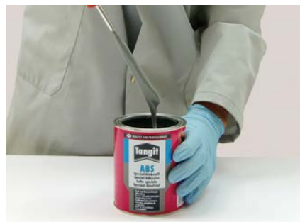
Checking the cement
